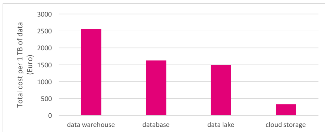
Figure 4: Comparing the total cost per one TB of data for each of data handling systems
