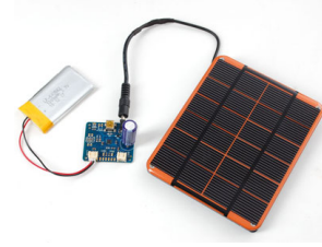
FIGURE 3.7: Example of a Solar Panel Circuit [37]
