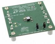
FIGURE 3.8: Full-wave bridge rectifier with a high efficiency buck converter optimized for high output impedance energy sources such as piezoelectric modules [38]
