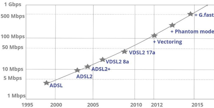
Figure 1-3 Evolution of DSL technology over time. The x-axis represents years, while the y-axis represents data. The graph shows how DSL technology has advanced over time, with increasing data rates enabling faster internet speeds for users: based on [14].
